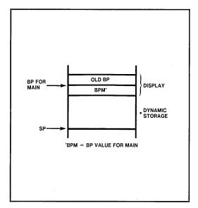
Figure 4-2a. Stack Frame for MAIN at Level 1
