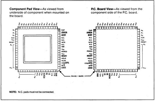
Figure 2. 80286 Pin Configuration
