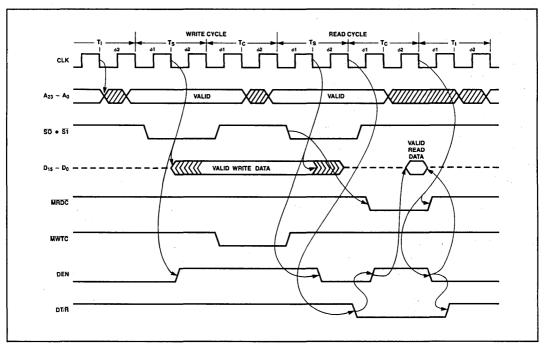
Figure 27. Back to Back Write-Read Cycles
