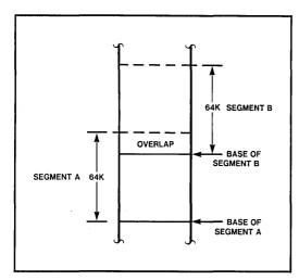
Figure 5-2. Overlapping Segments to Save Physical Memory
