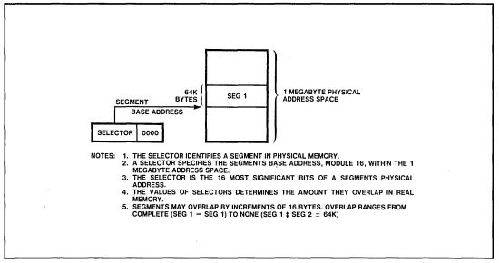
Figure 2-5. Real Address Mode Segment Selector Interpretation
