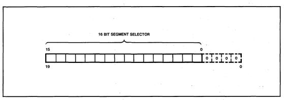
Figure 5-1a. Forming the Segment Base Address
