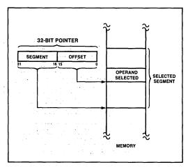
Figure 5. Two Component Address
