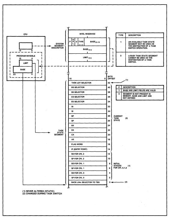
Figure 8-1. Task State Segment and TSS Registers
