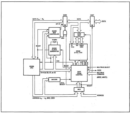
Figure 33. iAPX 286 System Configuration with Dual-Ported Memory
