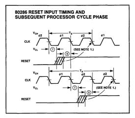
**NOTE 1:** When RESET meets the setup time shown, the next CLK will start or repeat  $\phi$ 2 of a processor cycle.
