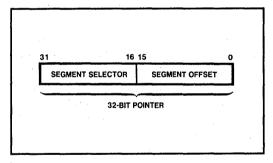
Figure 6-1. 32-Bit Virtual Address
