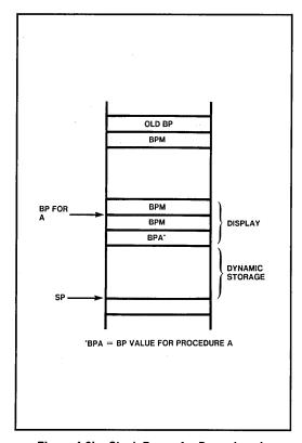
Figure 4-2b. Stack Frame for Procedure A
