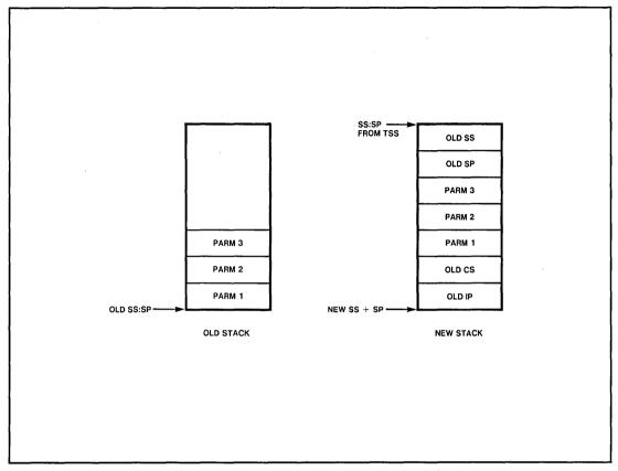
Figure 7-12. Stack Contents After an Inter-Level Call
