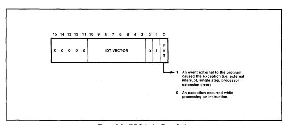
Figure 9-2. IDT Selector Error Code
