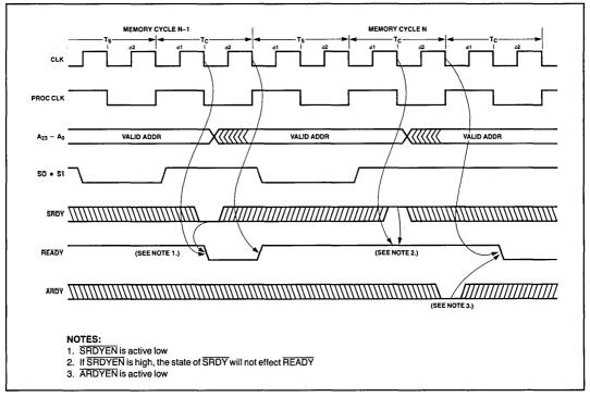
Figure 25. Synchronous and Asynchronous Ready
