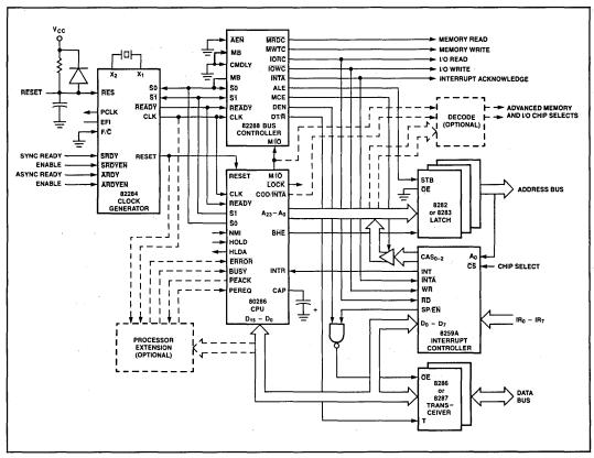
Figure 31. Basic iAPX 286 System Configuration
