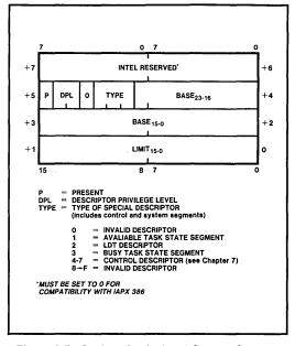
Figure 6-5. System Control and Special System Segment Descriptors
