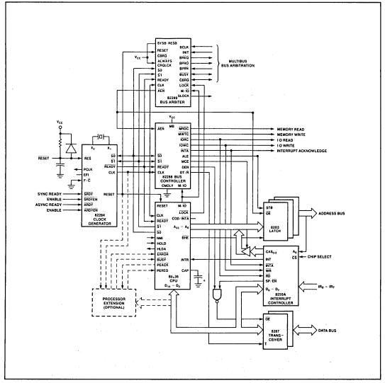
Figure 32. Multibus System Bus Interface
