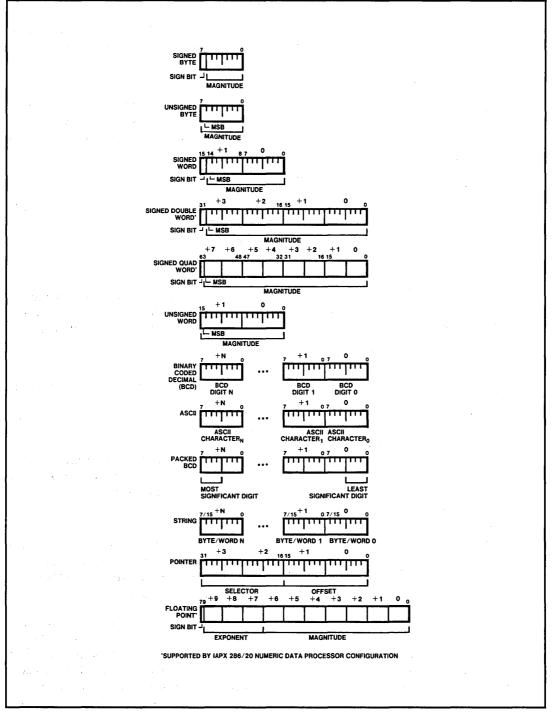
Figure 2-3. iAPX 286 Supported Data Types
