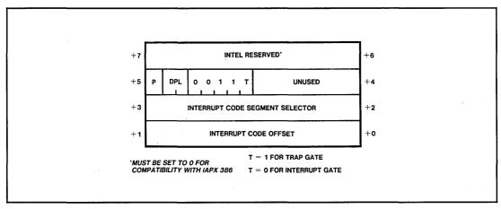
Figure 9-3. Trap/Interrupt Gate Descriptors
