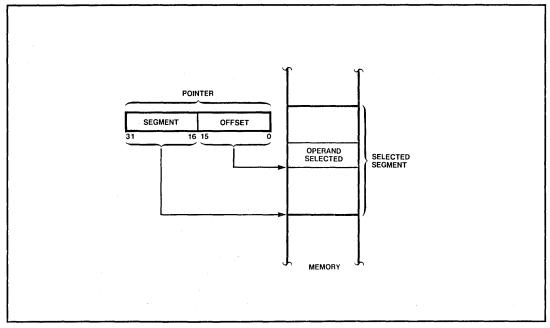
Figure 2-11. Two-Component Address
