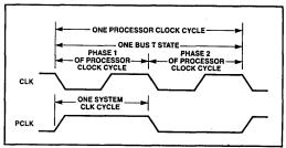
Figure 21. System and Processor Clock Relationships
