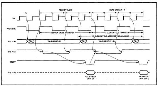
Figure 23. Basic Bus Cycle
