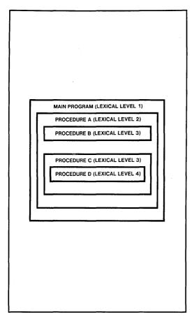
Figure 4-2. Variable Access in Nested Procedures
