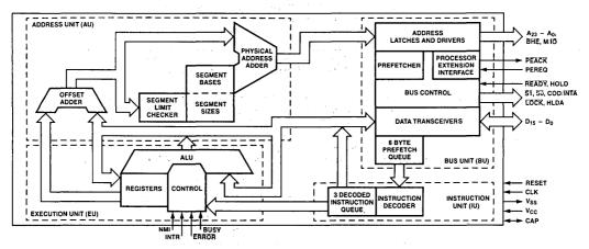
Figure 1. 80286 Internal Block Diagram
