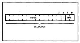
Figure 6-2. Format of the Segment Selector Component
