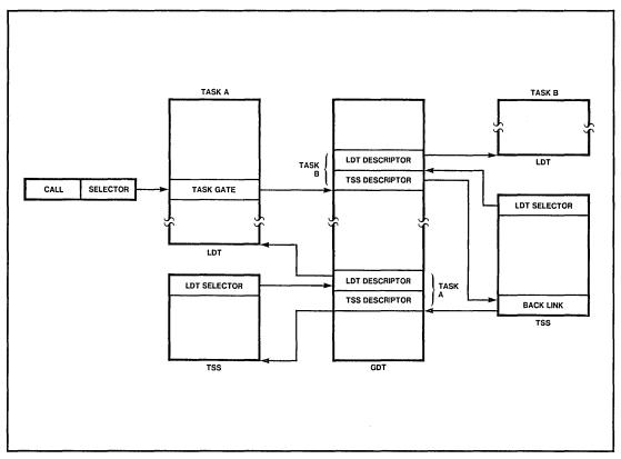
Figure 8-4. Task Switch Through a Task Gate
