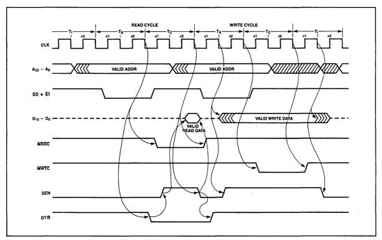
Figure 26. Back to Back Read-Write Cycles
