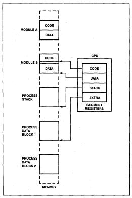
Figure 6. Segmented Memory Helps Structure Software
