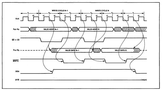
Figure 28. Back to Back Write-Write Cycles
