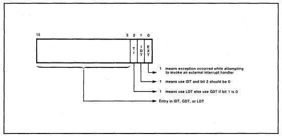
Figure 7-5. Error Code Format (on the Stack)
