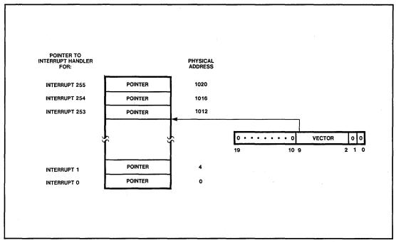
Figure 5-3. Interrupt Vector Table for Real Address Mode
