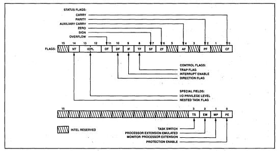
Figure 3a. Status and Control Register Bit Functions
