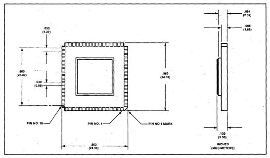
Figure 34. JEDEC Type A Package
