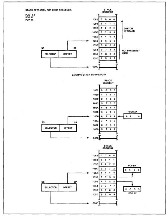
Figure 2-8. Stack Operation
