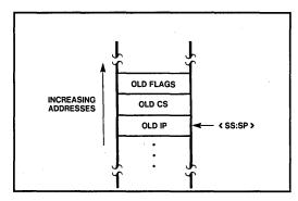
Figure 5-4. Stack Structure After Interrupt (Real Address Mode)
