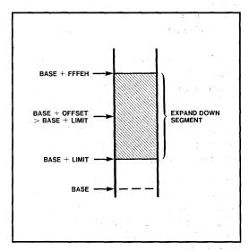
Figure 11-1. Expand Down Segment
