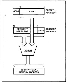
Figure 8. iAPX 86 Real Address Mode Address Calculation
