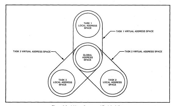
Figure 6-3. Address Spaces and Task Isolation
